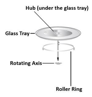
**CAUTION!** Never place the glass tray upside down. The glass tray should rotate smoothly. **CAUTION!** Both glass tray and Roller Ring assembly must always be used during cooking. **CAUTION!** All food and containers of food are always placed on the glass tray for cooking. **CAUTION!** If glass tray or turntable ring assembly cracks or breaks, stop using this appliance immediately, and please contact **Shun Hing Electric Service Centre Limited.**
